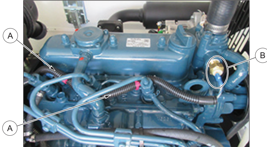
Figure 26 - Route Gray/Blue Wire to Coolant Temperature Switch
