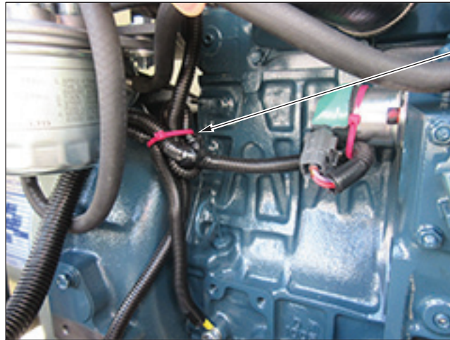
Figure 28 - Bundle and Cable-Tie Harness Wires
